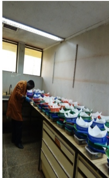
Extraction using modified Baermann technique (100ml soil & 5g fresh roots)- left 48hrs undisturbed.
